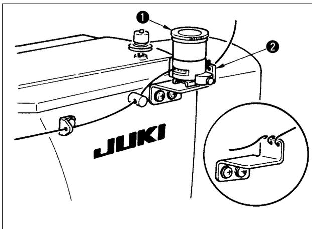
Fix silicon oil tank ① (MAXAP30EX00) with the magnet.
