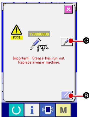
When error "E221 Grease-up error" is displayed, be sure to replenish the designated places below with grease. Then call the memory switch U245, press CLEAR button **C** **A** and set NUMBER OF STITCHES **D** to "0".
