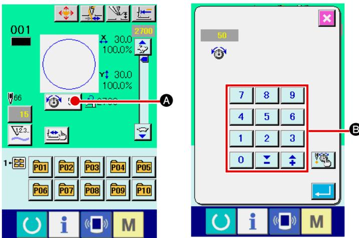
1) Select THREAD TENSION button
