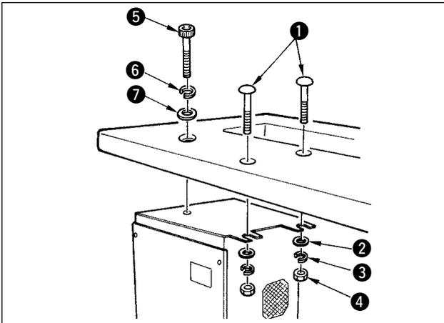
Install the electrical box on the underside of the table at the location illustrated using round-head bolt **1**, plain washer **2**, spring washer **3** and nut **4** supplied with the machine, and using bolt having hexagonal indentation on the head **5** spring washer **6** and plain washer **7** supplied with the machine.
