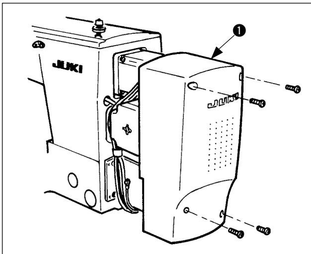
Install motor cover ❶ on the machine main unit with screws supplied with the machine as accessories.
