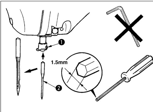
Loosen setscrew ① and hold needle ② with the long groove facing toward you. Then fully insert it into the hole in the needle bar, and tighten setscrew ①.
