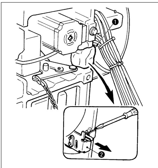
Remove tape ② fixing the lever section of safety switch ①.
