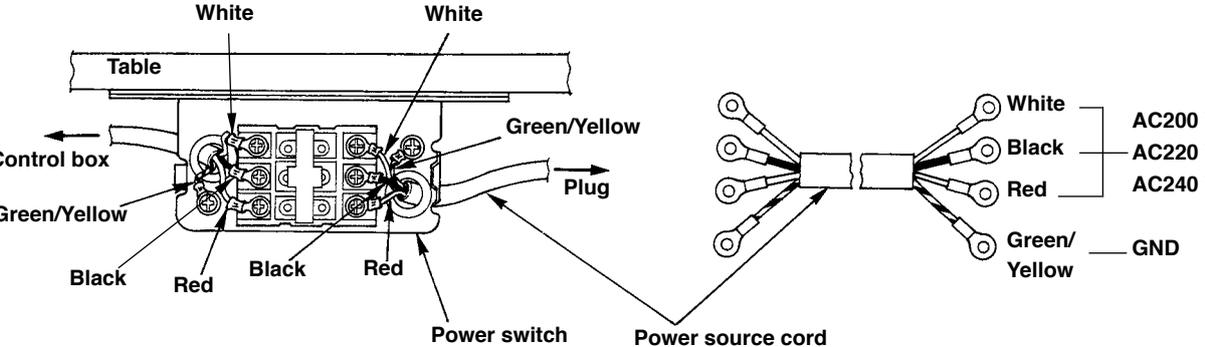
**3-3. Installation of the sewing machine head**
