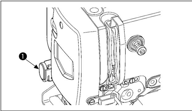
When TEMPORARY STOP switch ① is pressed during sewing, the sewing machine can be stopped. At this time, the error screen is displayed to inform that the stop switch has been pressed.
