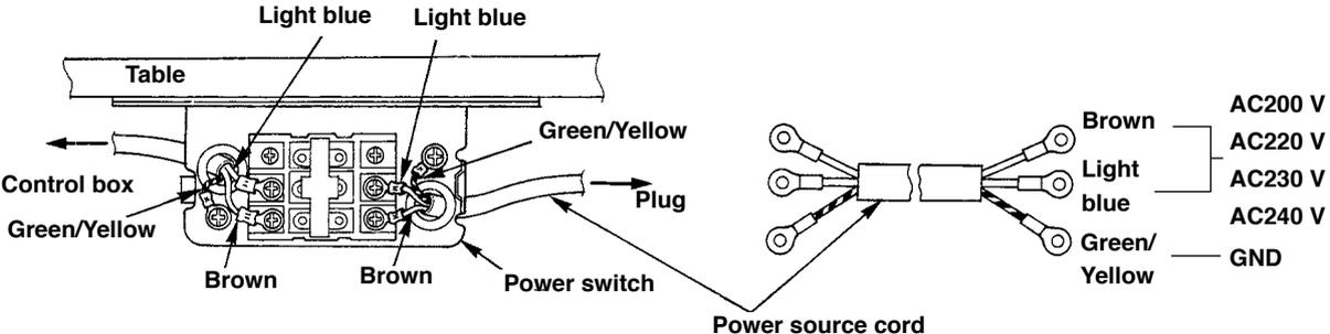
**• Connecting three phase 200V, 220V and 240V**
