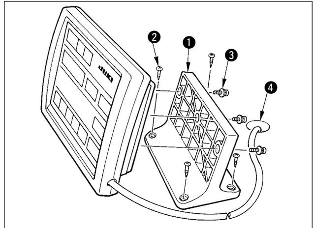
Fix operation panel installing plate ① to an optional place on the table with wood screws ②, and pass the cable through table hole ④. Fix the operation panel on panel installing plate ① with screws ③ supplied as accessories. Fix the cable on the bottom surface of the table with the staples supplied with the machine as accessories.
