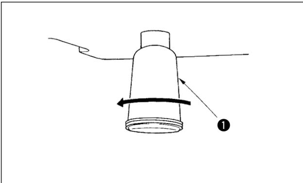
When polyethylene oiler ① becomes filled with oil, remove polyethylene oiler ① and drain the oil.
