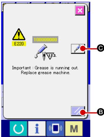
When the sewing machine has been used for a certain number of stitches, error "E220 Grease-up warning" is displayed. This display informs the operator of the time of replenishing the designated places with grease. Be sure to replenish the places with the grease below. Then call the memory switch U245, press CLEAR button **C** **A** and set NUMBER OF STITCHES **D** to "0".
