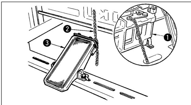
Connect the machine ① and manual pedal ③ with chain ②.
