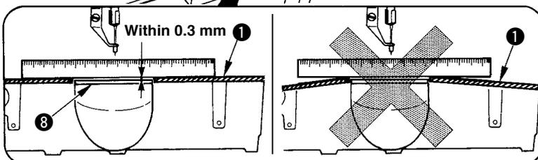
1. Be careful so as not to mistake the direction of throat plate auxiliary cover support.
