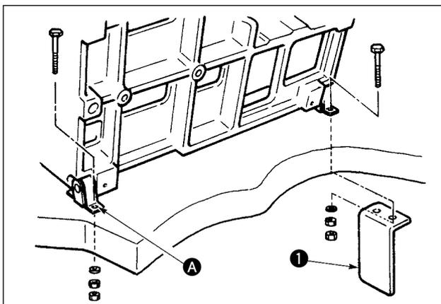
1) Fit the holes of hinges **A** to the holes of table and fix as shown in the figure.
