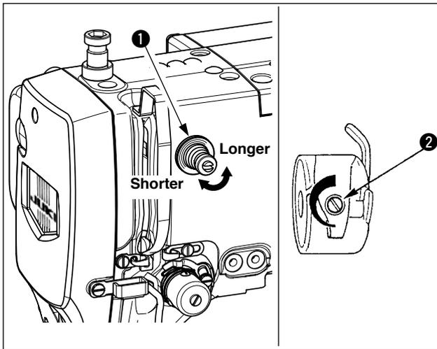
If thread tension controller No. 1 ❶ is turned clockwise, the length of remaining thread on the needle after thread trimming will be shorter. If it is turned counterclockwise, the length will be longer. Shorten the length to an extent that the thread is not slipped off.
